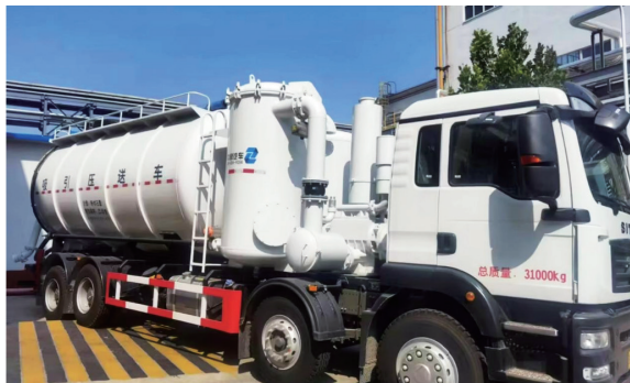
Figure 5-11 Vacuum Tanker Truck
