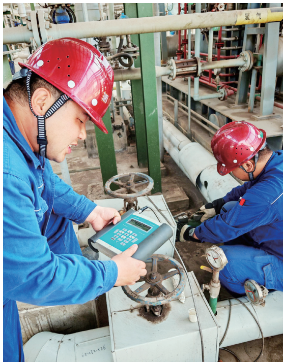
Figure 5-8 Water System Audit Organized by the Group's Laoting Base Using the "FLUXUS F60X" Online Flow Meter
